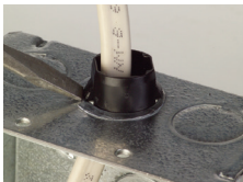
Easy Removal - Push the wing tab of the connector with a screwdriver. Push the connector through the knockout towards the inside of the box.
